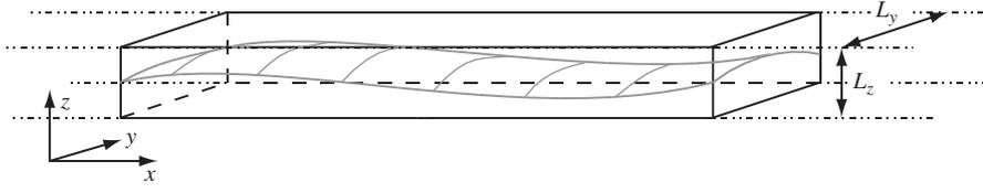
Figure 2.2: EM waveguide with rectangular cross-section. The structure of the eigenmodes of the EM field is determined by boundary conditions at the walls of the cavity.
