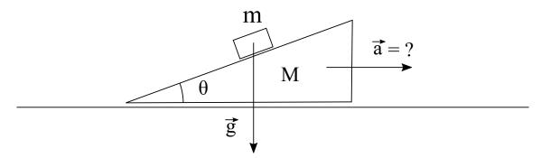
A wedge with mass *M* can slide without friction along a floor, and on the wedge there is a block of mass *m* that also can slide without friction. Imagine that we initially hold both the block and the wedge at rest, and then suddenly release them. The block is affected by gravity, and by a normal force from the wedge. (The wedge is kept on the surface by a normal force from the floor.)
