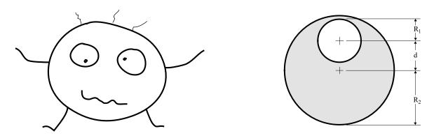
To the left is displayed a realistic representation of object Å. This body has total mass M, and is accurately approximated by a sphere of radius  $R_2$  with uniform density, wherein there is a spherically shaped cavity (up towards the head) containing absolute vacuum. This spherical cavity has radius  $R_1$ , and its center is displaced by a distance d from the center of the large sphere. We have  $R_2 \ge R_1 + d$ , i.e., the cavity lies completely within the larger sphere.
