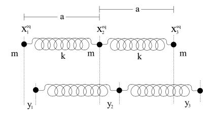
The motion of particles that interact harmonically can be decomposed into especially simple components, the *normal modes*. For each such normal mode, the particles perform a collective periodic motion with respect to one single frequency.
