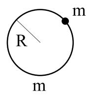
Consider an infinitely thin ring of mass m and radius R. On the ring there is an additional point mass m attached (hence the total mass is 2m). Determine the inertia tensor with respect to the principal axis system with origin at the center of mass.
