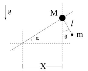
A mass *M* slides without friction along a straight rail that is tilted at a fixed angle  $\alpha$  with respect to the horizontal plane. From the mass *M* hangs a pendulum in the form of a massless rod of length *l* to which a mass *m* is attached. The pendulum only swings in the plane of the vertical axis and the rail. Both the mass *M* and *m* are affected by the constant gravity *g* in the vertical direction.
