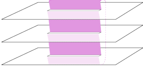
Figure 2.4.: Sketch of the Riemann surface for \alpha = 3 on which the path integral has to be computed. Periodic boundary conditions are assumed for one dimension of the white sheets representing the copies of part B . The pink sheets constitute the surface on which the path integral of part A is evaluated. ©P. Calabrese.
