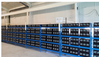
Figure 1.6: Left: Cryptocurrency mines consists of racks of computers that try random inputs hoping to find a solution to a mathematical puzzle. Right: If you can do better, there’s 300b dollars on the table (as of early 2023). Credit: Wikipedia, Statista.
