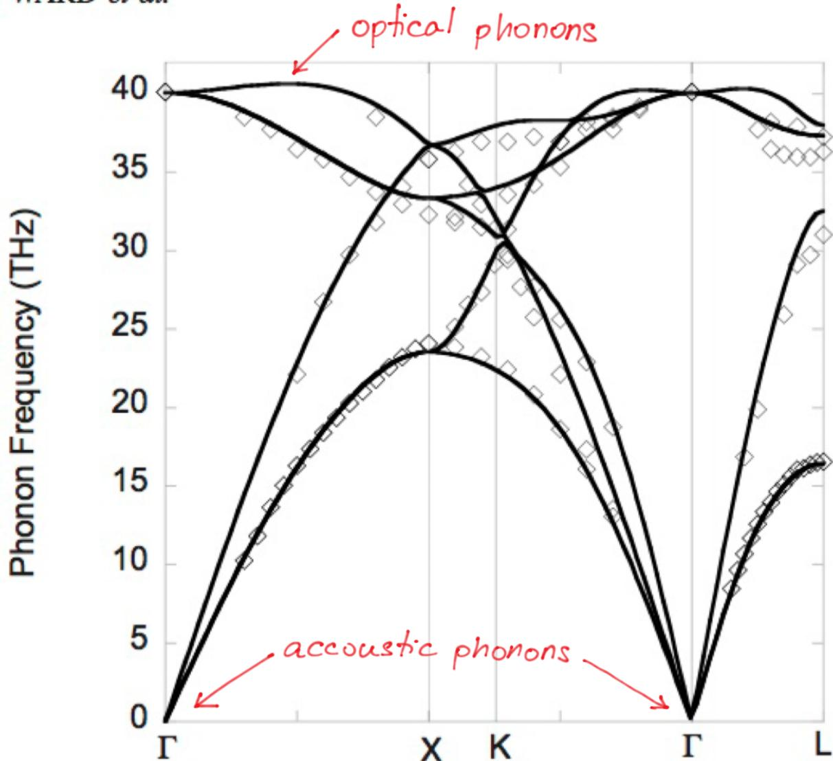
FIG. 1. Phonon dispersions of diamond. *Ab initio* calculations (solid line) and experiment (open diamonds).
