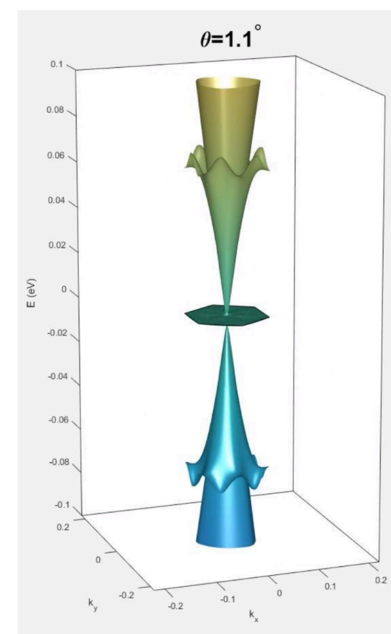
electronic band structure with a **flat band** in twisted bilayer graphene
