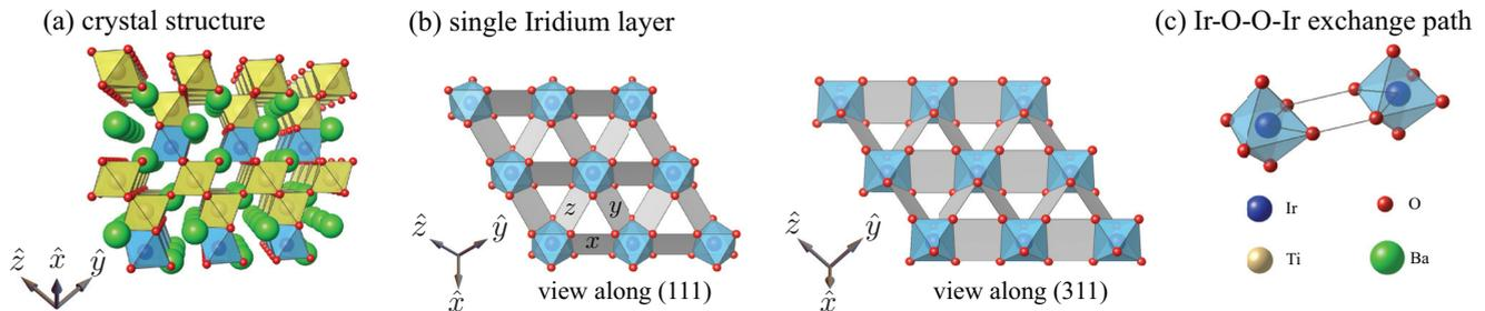
FIG. 1. (Color online) (a) Crystal structure of  $\text{Ba}_3\text{IrTi}_2\text{O}_9$ . (b) View of single iridium layers from two different perspectives. Within the plane, the  $x$ ,  $y$ , and  $z$  exchange paths are indicated by the gray planes. The planes labeled by  $x$  ( $y$ ,  $z$ ) are normal to the coordinate axis  $\hat{x}$  ( $\hat{y}$ ,  $\hat{z}$ ). (c) The exchange between the iridium moments (blue) is mediated by two coplanar exchange paths.
