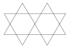
The Kagome lattice consists of a regular arrangement of corner-sharing triangles, as shown in the figure. The lattice points are the corners of the triangles.
