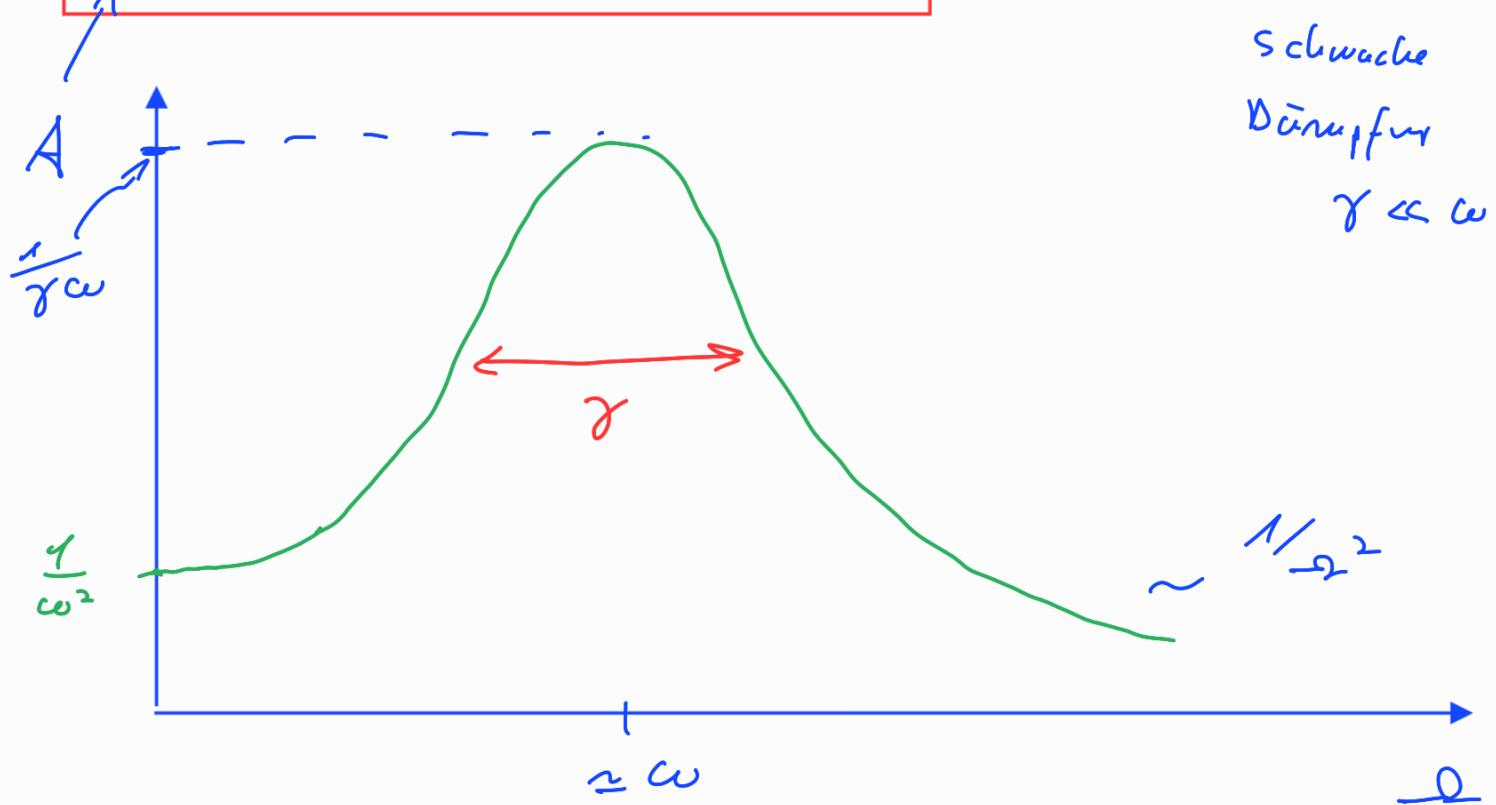
$$\frac{\alpha}{f_0} = \frac{1}{\omega^2 - \omega^2 + i\gamma\omega}$$
