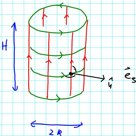
$$\varphi, z \mapsto \vec{S}(\varphi, z) = \begin{pmatrix} R \cos \varphi \\ R \sin \varphi \\ z \end{pmatrix}$$
