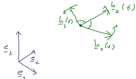
$$\text{aus } \underline{h}_i(t) = D(t) \underline{e}_i \quad \text{folgt} \quad \dot{\underline{h}}_i = \dot{D} \underline{e}_i \\ = D D^T \dot{D} \underline{e}_i$$
